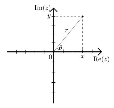
As seen on the diagram above, the modulus, r, refers to the distance from the point representing the complex number to the origin. Meanwhile, the argument,  $\theta$ , refers to anticlockwise angle the positive x-axis makes with the line from the origin to the point.
