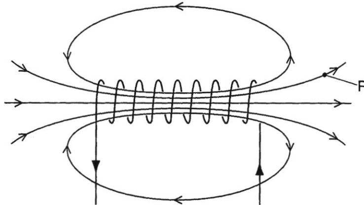
What is the effect on the magnetic field at the point P of using a larger current in the opposite direction?
