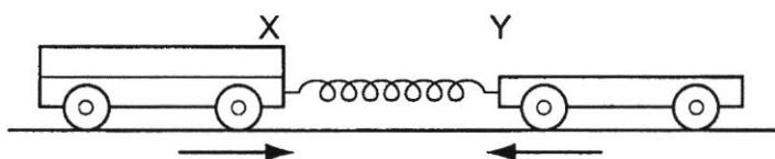
When the trolleys are released, the initial acceleration of X is  $2 \text{ m/s}^2$  to the right.
