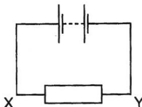
What are the directions of the conventional current flow and electron flow through the resistor?
