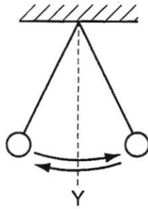
The first time the pendulum passes through Y, a stopwatch is started. The twenty-first time the pendulum passes through Y, the stopwatch is stopped. The reading is  $T$ .
