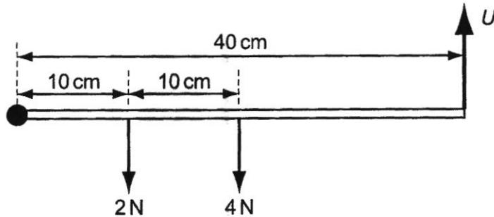
An upward force  $U$  is needed to keep the beam horizontal.
